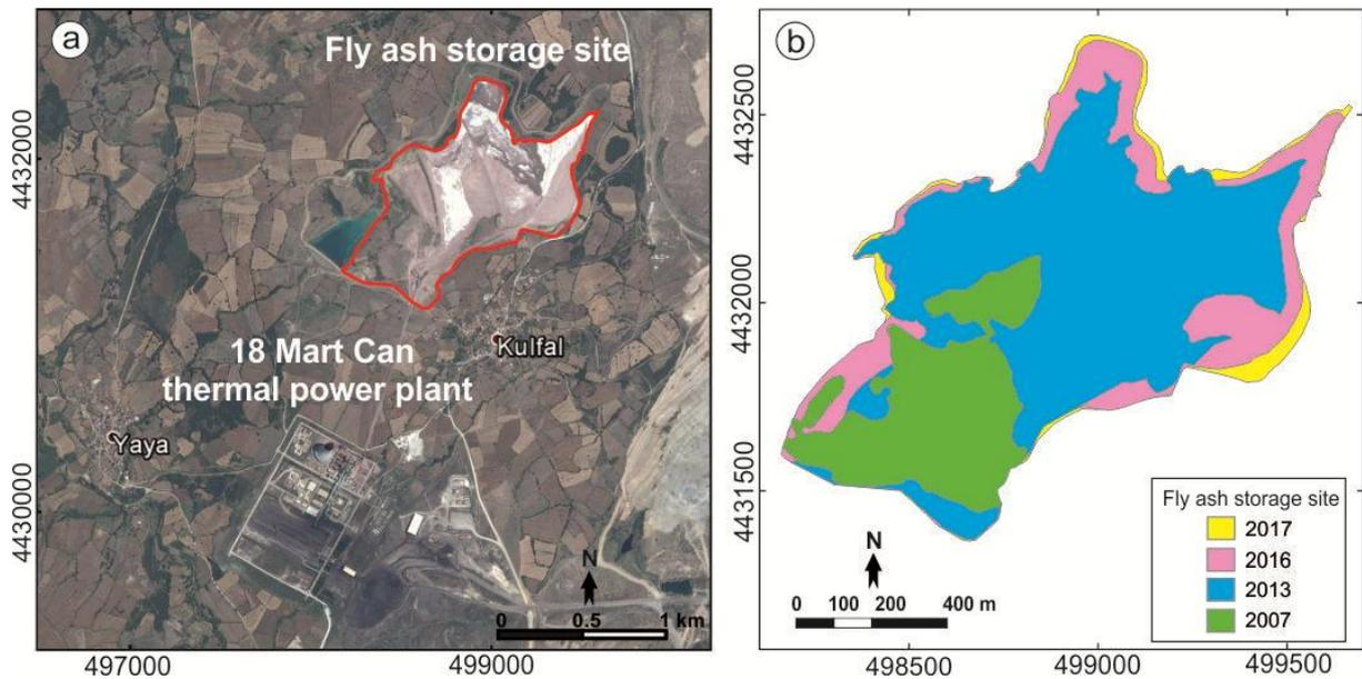
**Figure 2a.** 2017 year Google earth satellite image from 18 Mart Can Thermal Power Plant **b.** Areal change of fly ash storage site in time period.
